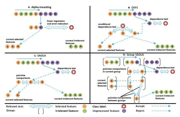
**Fig. 2:** Illustrating examples of the four relevant feature selecting processes that operate on Feature 6 of a set of nine features arriving one by one using four online streaming feature selection methods. "Current selected features" is the temporary relevant features which have been selected currently. "Current irrelevant features" is the irrelevant features which have been rejected by the relevant test.
